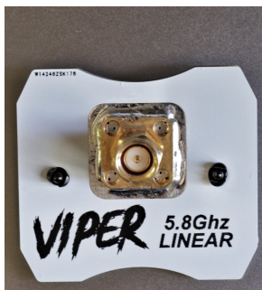
Back side, SMA connector
