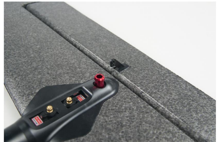
Install the horn chuck onto Horizontal tail as the same way as aileron.
