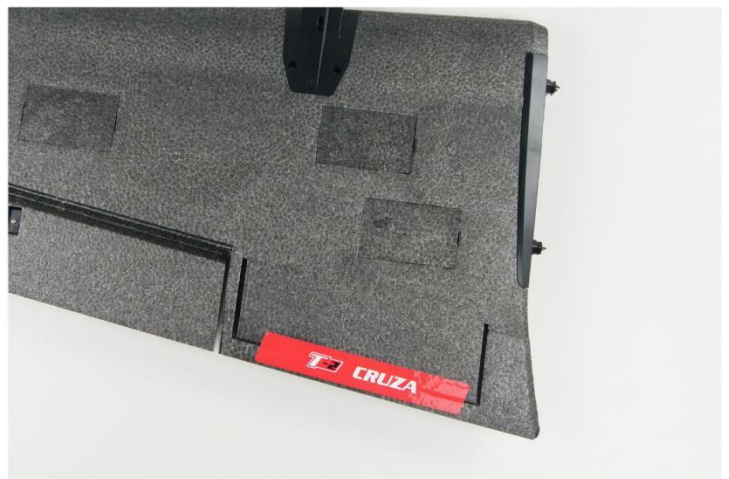
Apply the sticker over the flap opening ( When flaps are not installed) to prevent airflow-induced vibration of the flap control surface during flight.
