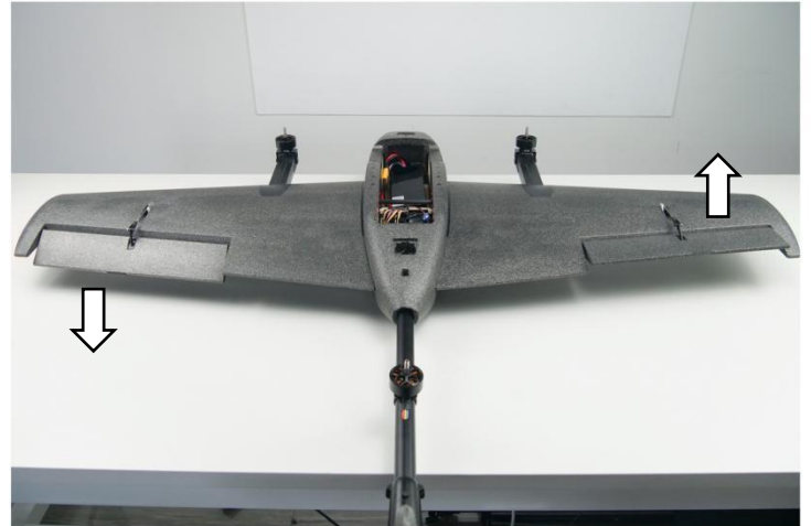
The left aileron should be downward, the right aileron should be upward.
