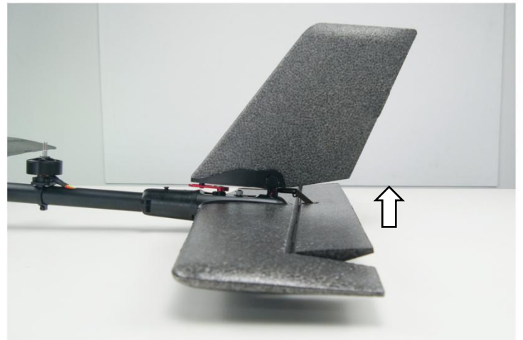
The horizontal tail control surface should be upward.
