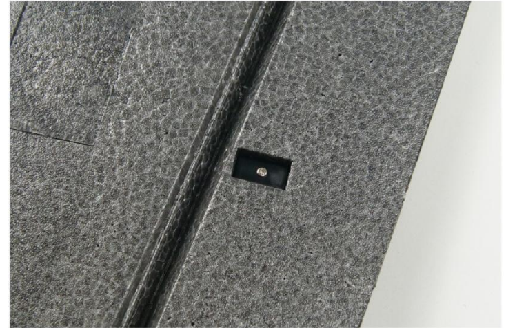
On the reverse side, install the horn buckle and secure with PA2*6 screws.
