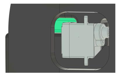
5. Push in the servo while pulling the servo wire further out
