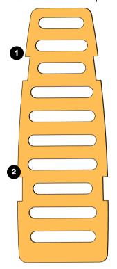
2. Apply glue on the complete bottom surface area o the base plate
