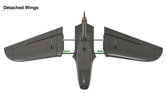
4. Pull the carbon rods out of the main body
