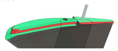
6. Push the lower stabilizer in to the main body and hold it till the glue is cured
