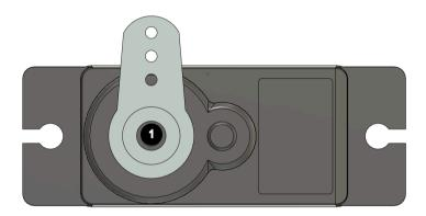
2. Widen the hole for the push-rod in the servo horn
