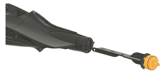
6. Dry-fit the installed motor mount with the two rods holding it in place
