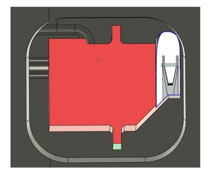
4. Feed the servo cable through the wings wire channel while installing the servo
