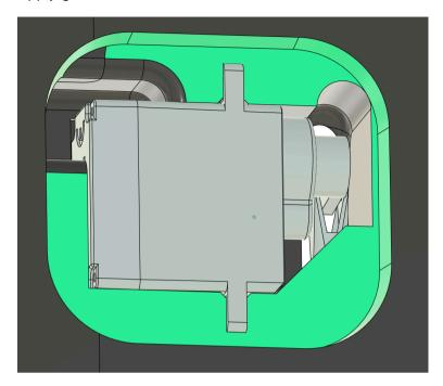
7. Attach the cover and fixate it with some weight will the glue is cured
