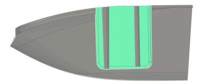
2. Push the lower stabilizer and the cover together and hold it till the glue is cured
