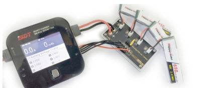
Charging board connected to a charger
