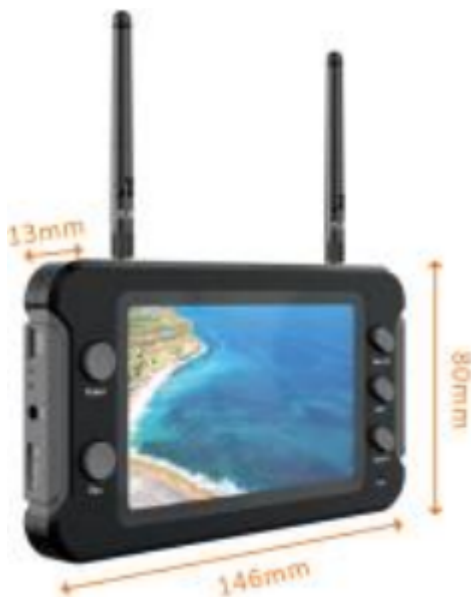
Device dimensions: 146 × 80 × 13 mm (antennas not included)
