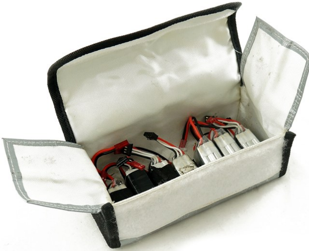
The bag opened. Inner lining of glass-fibre fabric, white insulating fibres visible at the cut edge, polyester edge binding and hook-and-loop fastener.
