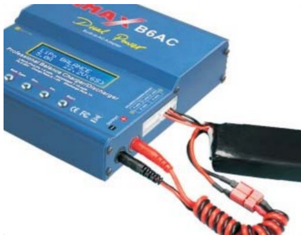
Correct battery connection for balance charging
