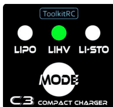
Charger switched on, LIHV type selected
